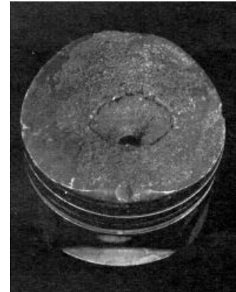
Pre-ignition Damage (Hastings)
