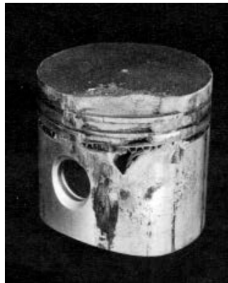
Detonation Damage (Hastings)
