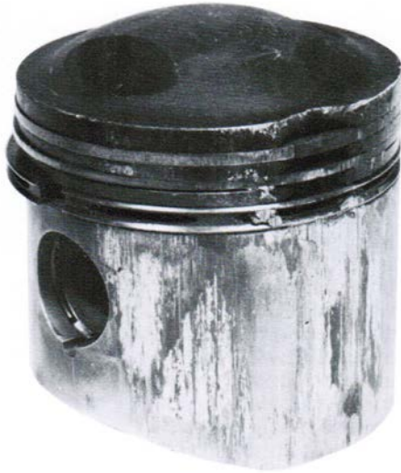
Mahle Fig 1-3 Detonation Damage
